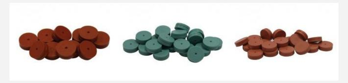
The Greyhound Chromatography range of Premium GC Septa are precision-moulded and available with a recess on the injection side, to guide the syringe needle to the same point with every injection. The Centre Guide design requires less force for initial penetration for a smoother feel. Septum life may be enhanced in some applications by minimizing tearing and coring.
